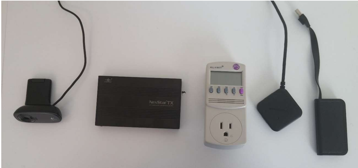
FIGURE 3: THE PERIPHERALS USED IN THE EXPERIMENTS, FROM LEFT TO RIGHT: C310 LOGITECH WEBCAM, FUJITSU HARD DRIVE, POWER METER, TWO USB ROOT HUBS
