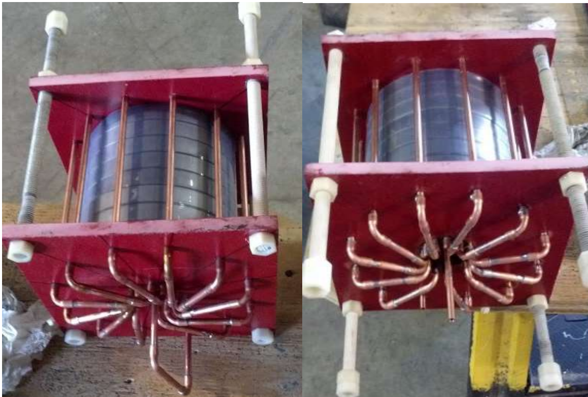
Figure 5.4 Photograph of the 12-turn MnZn saturating switch.
