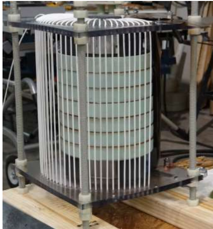
Figure 5.5 Photograph of the final build of the pulsed primary switch.
