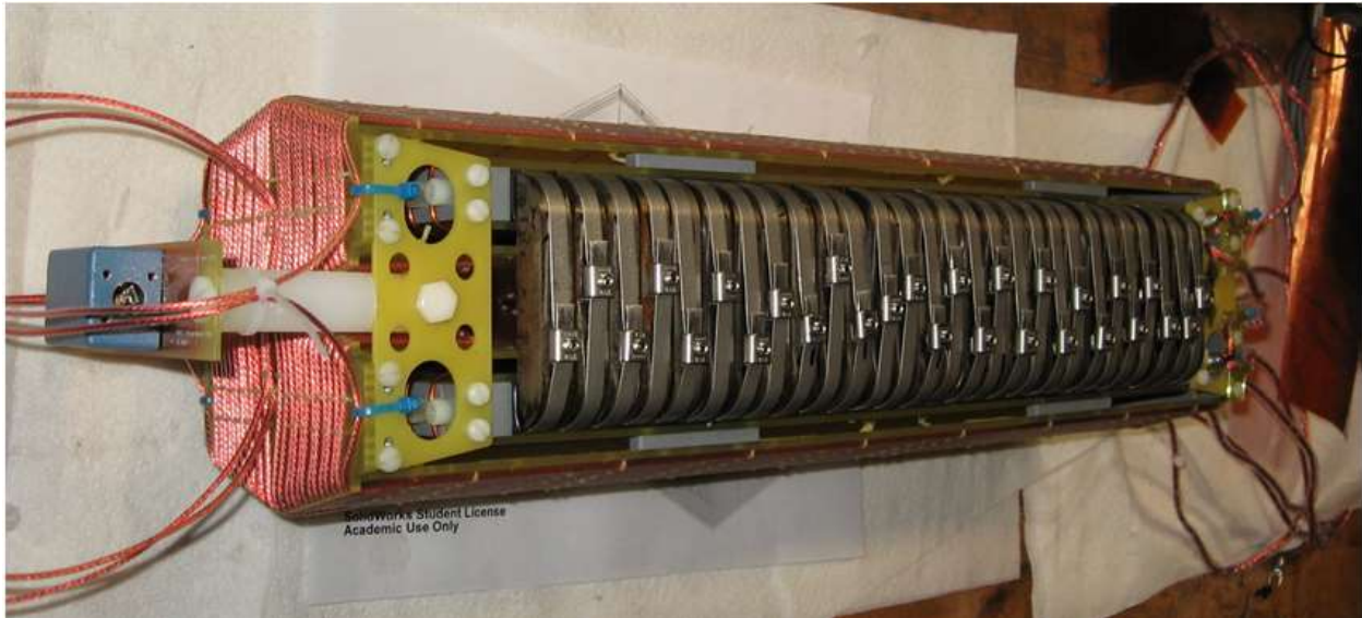
Figure 5.1 Final build of the saturating transformer.
