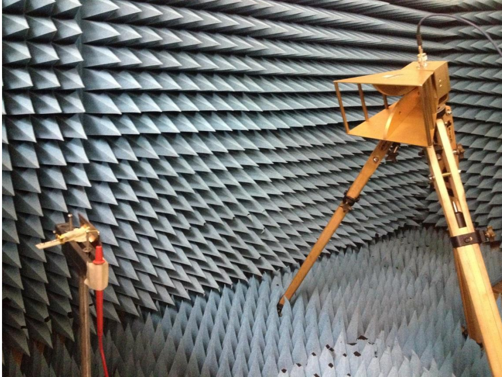
Figure 4.27: A photograph of the setup used to test the broadband rectenna design.
