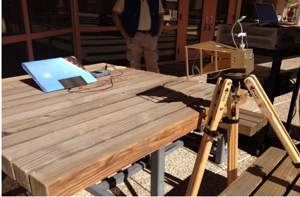
Figure 5.1: Photograph of the setup for the measurements recorded on the effects of a rectenna on a solar cell
