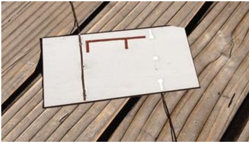
Figure 5.6: Photograph of the PIFA placement on the back of a solar cell.
