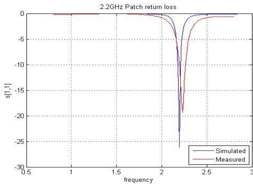
Figure 3.17: Measured S_{11} parameters for the fabricated patch antenna.
