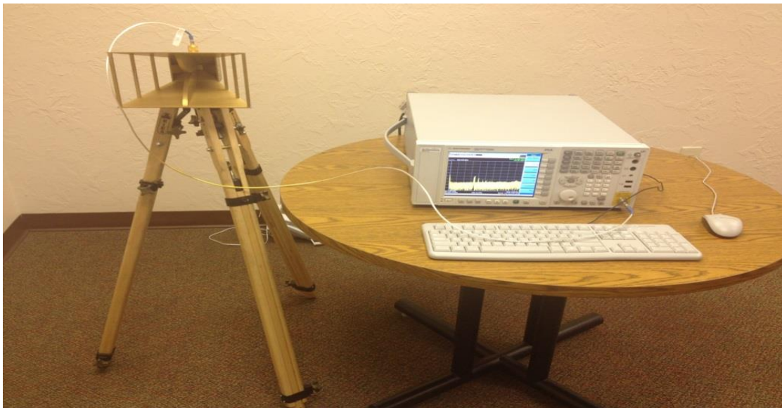
Figure 3.2: Setup for spectrum analyzer measurements.
