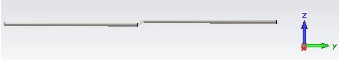
Figure 32: Half-Wave Dipole With Intentional Offset
