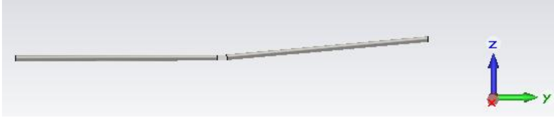
Figure 34: Half-Wave Dipole with Intentional 5° Offset.
