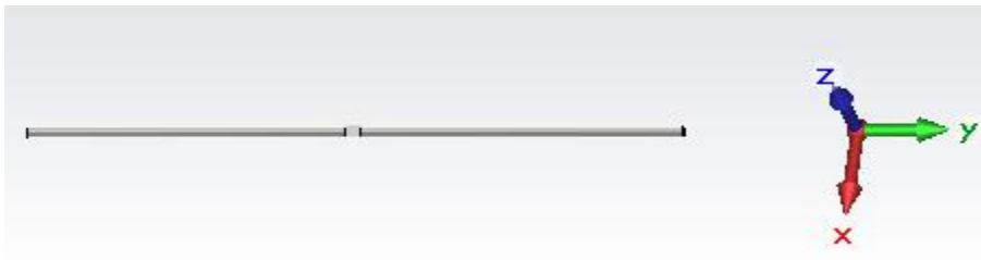
Figure 29: Resonant Half-Wave Dipole Model.
