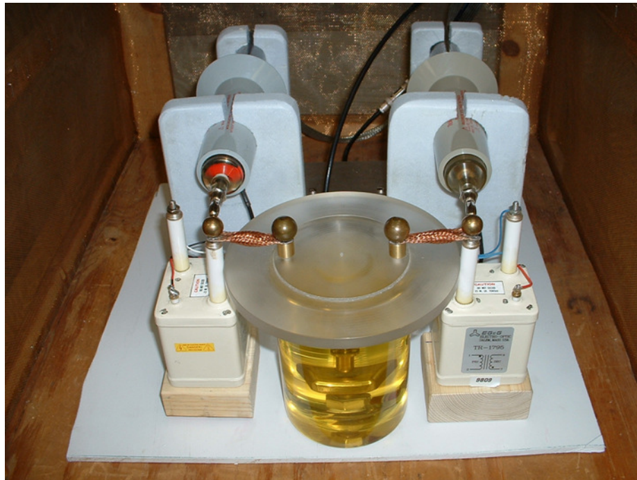
Fig. 4.2: Photograph of chamber, transformers, and probes.
