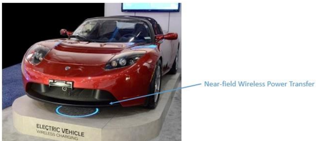
Figure 83: Near-field wireless power transfer - electric vehicle using wireless charging in the near field [4].
