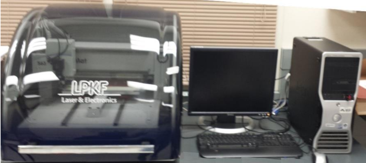
Figure 71: LPKF Milling Machine
