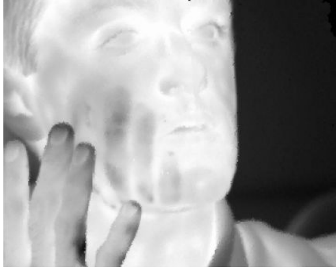
Figure 3.12 Thermal image taken with at 77 K with and integration time of 16.3 ms and using a two-point non-uniformity correction
