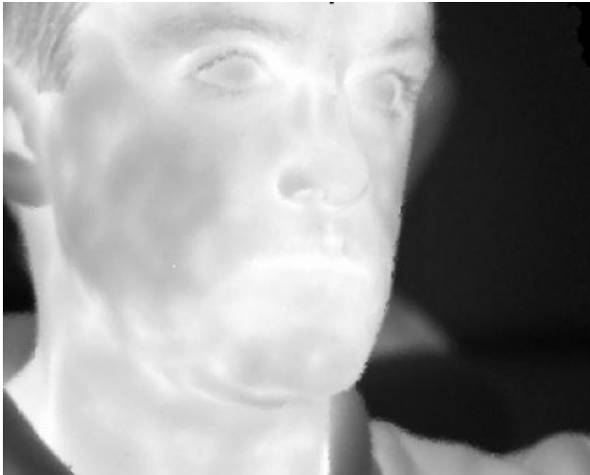
Figure 5.1 MWIR image captured from the first SL nBn FPA with a non-uniformity correction applied at T = 77 K with a NETD = 26mK
