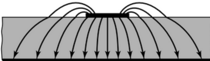
Figure 3-2: Electric Field Lines From Microstrip [22]
