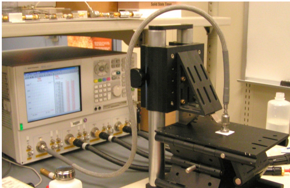
Figure 2-5: Dielectric Probe Set-Up
