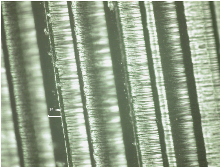
Figure 5-20: Sr-90 Radiated (3 Days) ABS Under Microscope
