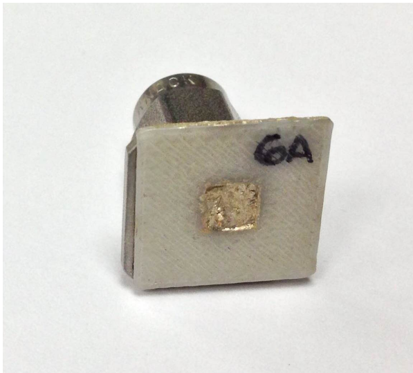
Figure 3-15: 25 GHz Antenna With Conductive Paint
