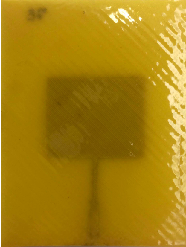
Figure 4-6: The back of a 5 GHz antenna coated with Kapton tape
