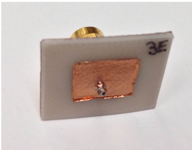
Figure 3-19: 10 GHz Antenna Made With Copper Tape And Solder
