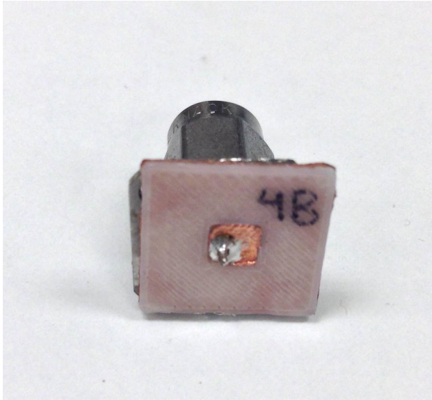
Figure 3-18: 25 GHz Antenna Made With Copper Tape And Solder
