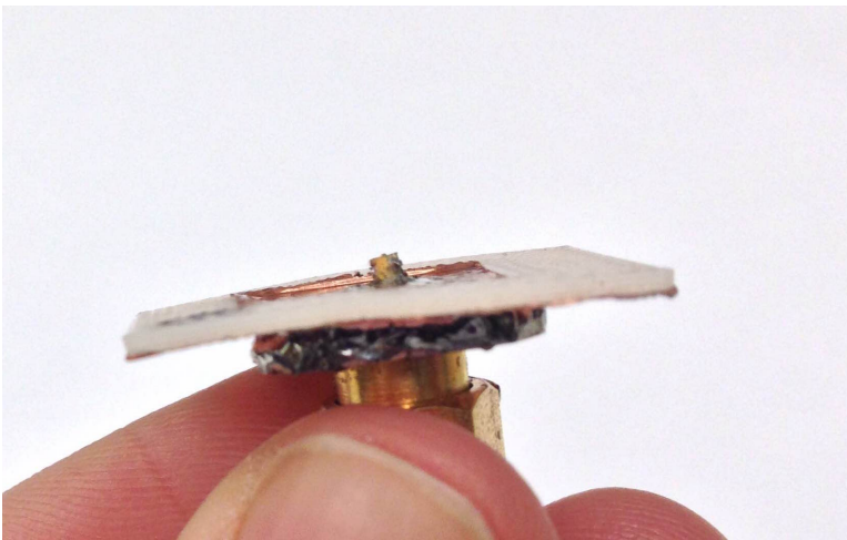
Figure 3-17: 10 GHz Antenna Warped From Soldering Heat
