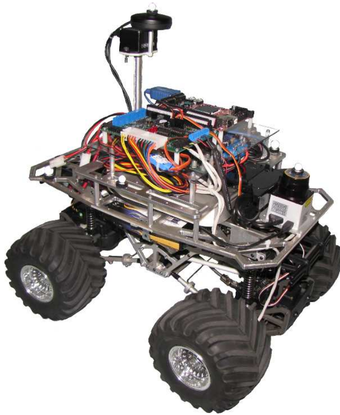
Figure 3.3: The TXT-1 Robot with the mounting hardware, plates and electrical systems.
