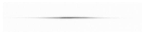
Figure 5.7: Doppler beam profile for cooling the ring of ions. The beam size at the waist is on the order of 100  $\mu$ m by 3000  $\mu$ m.
