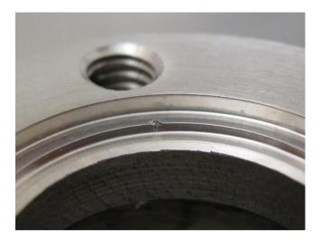
Figure E.1: Knife-edge damage on a custom ordered, unused CF component.
