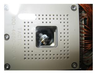
Figure 3.23: Calcium oven aligned. A microscope glass slide is covering the cut-out of the ZIF socket. The oven barrel (the same construction shown in Fig. 3.21a but equipped with spread-limiting tube), viewed form the top, is positioned as desired. Once sublimated, Ca deposits on the slide and a thin metallic film can be seen at a facilitating angle. The spot was not captured with the camera despite some effort.
