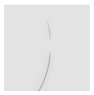
Figure 5.10: Chain in the ring trap before correction. The segment shown corresponds to what is at 12 o'clock in Fig. 5.9b. The gap in the chain is due to the loading hole potential bump.
