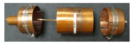
Figure 3.10: Helical resonator details, side view. The antenna (cap on the right) and endcap (on the left) slide onto the shield around the helix (middle).
