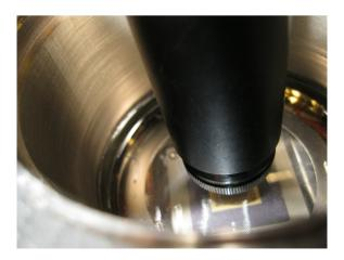
Figure 5.5: Installed device with the screening mesh on the re-entrant viewport.
