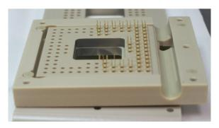
Figure 3.16: ZIF socket re-assembly after cleaning. The cam shaft, screws, pins, and PEEK body parts are processed as regular UHV parts.
