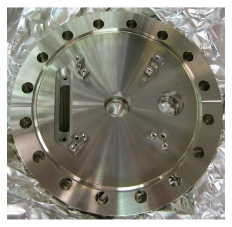
Figure 3.6: Custom 6" CF bottom flange with attached support posts, vacuum side. The 100 pin Micro-D connector is on the left, the cut-outs are for standard 1.33" flanges (for the atomic oven in the center, and a spare) on air side.
