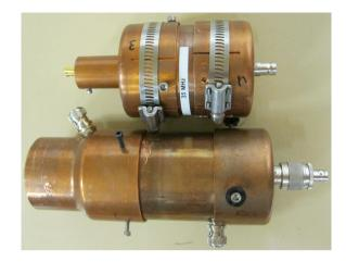
Figure 3.9: Typical implementations of quarter wave helical resonators at SNL.
