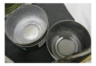
Figure 3.20: Calcium oxidation. The can on the left hand side has been stored opened in a dry box that turned out to not provide enough oxygen displacement, hence almost all calcium inside has oxidized (CaO is off-white in appearance). The can on the right hand side is freshly opened (less than 5 minutes exposure to air), but oxidation is already seen from the color of the finest particles.
