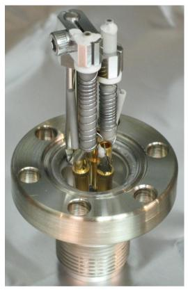
(b) Atomic oven for two species, Yb and Ca, after  $\sim 3$  years of use. Spread-limiting tubes on top are in place.
