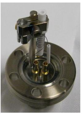
(a) Atomic oven with an extra joint for precise barrel alignment. The spread-limiting tube on top is not in place yet.
