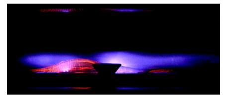
Figure 6.9: Mesh screen damage during plasma generation. Argon plasma is seen as the cloud with a purple/pink hue. The red/orange bulge is a heated and deformed mesh screen similar to the one covering the viewport in Fig. 5.5.
