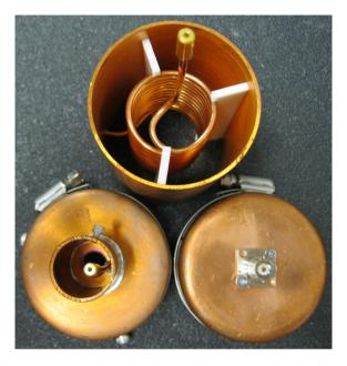
Figure 3.11: Helical resonator details along the axis. The helix is supported by the shield via Teflon slabs (top). A shield extension and ground wire are soldered to the endcap (bottom left). The antenna is equipped with a BNC connector (bottom right).
