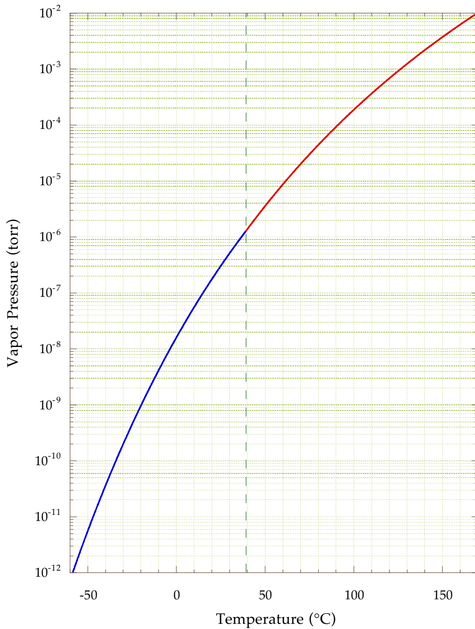
Figure A.2: Rubidium vapor pressure as a function of temperature.
