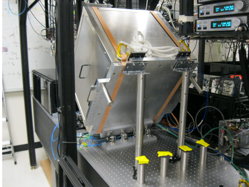
Figure 6.4: Picture of the interferometer subjected to variations in the orientation of gravity. A winch bears the approximately 100 kg load of the apparatus as it is secured. Not shown: One incredibly nervous graduate student.
