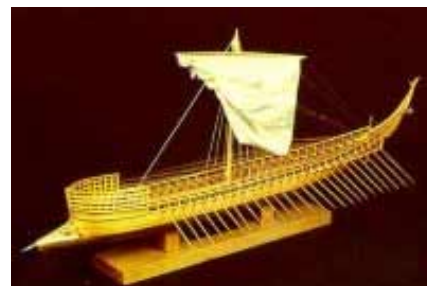
Figure 1.2: Model of a penteconter, a galley with one row of oars on each side.
