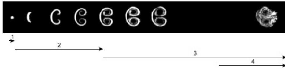
Figure 2.5: Stages of the evolution of an RMI-driven flow evolving from initially diffuse, nearly 2D cylindrical initial conditions. Flow direction is from left to right. The dark field corresponds to lighter gas. 1 - initial nearly-linear perturbation growth, 2 - deterministic vortex-dominated growth, 3 - onset of secondary instabilities and emergence of disordered elements in the flow, 4 - transition to turbulence [16].
