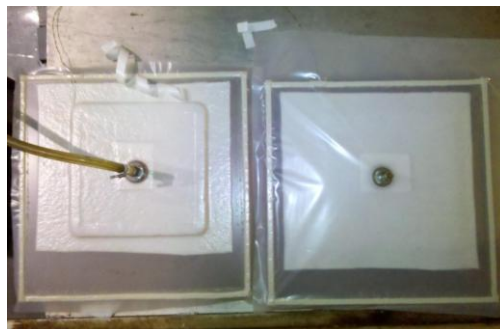
Figure 3-14: Vacuum drawn on sealed panels prior to cure
