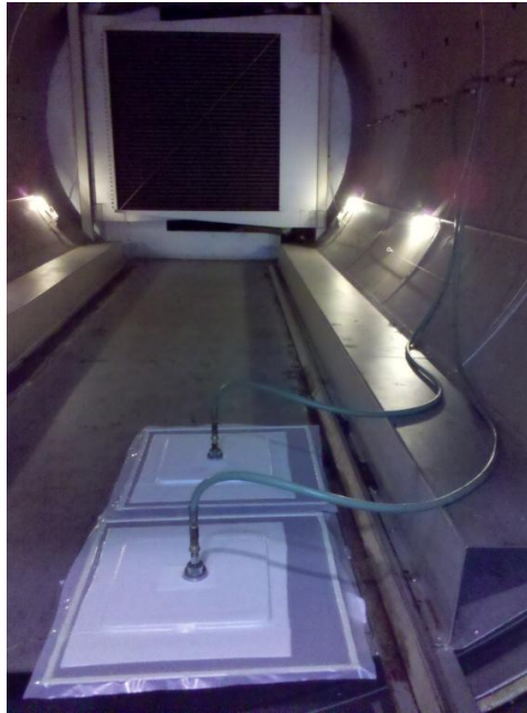
Figure 3-15: Panels ready for cure in autoclave
