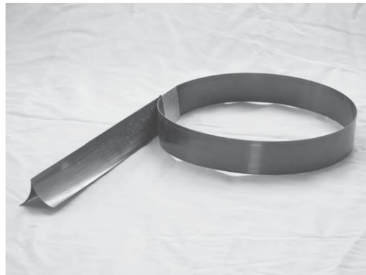
Figure 2-3: Partially rolled Triangular Rollable And Collapsible (TRAC) Boom
