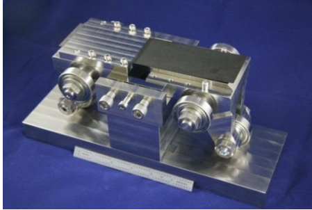
Figure 3-18: Carts in the alignment fixture with one of the sample covers removed
