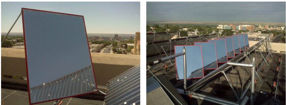
Figure 2.10: Photos of mirrors set at \alpha = 20^\circ and \beta = 42^\circ in front of the solar vacuum tube collectors
