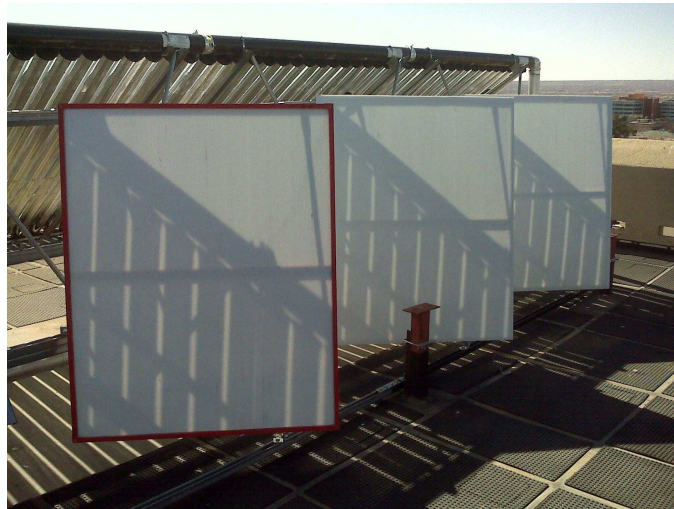
Figure 2.8: From right to left: 1 st prototype (Aluminum Frame), 2 nd prototype (Pressure Treated Lumber Frame), 3 rd prototype (Regular lumber made into a slotted frame)
