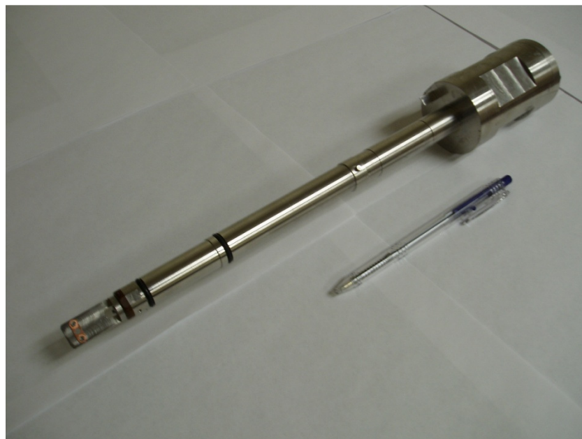
Figure 12: Custom manufactured TEM holder
