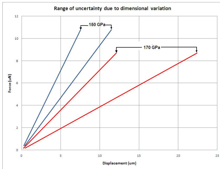
Figure 30: Range of uncertainty in actuator response with elastic modulus 150 – 170 GPa
