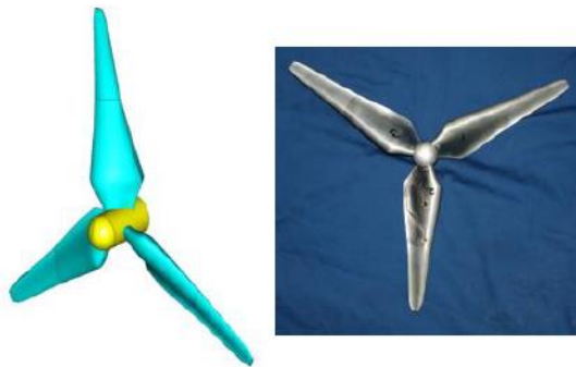
Figure 2: Sandia turbine CAD geometry and manufactured turbine [8]
