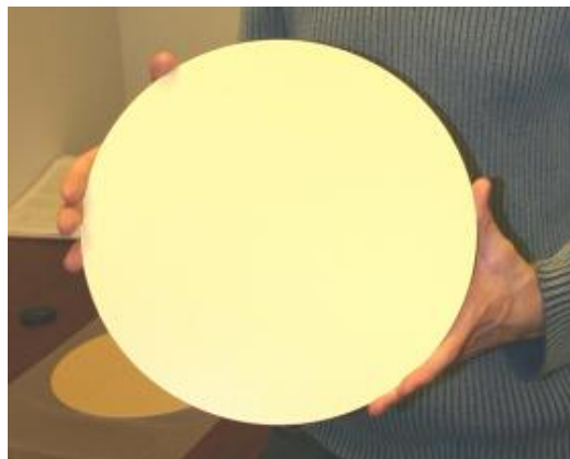
Figure 50. Flat-plate microwave lens. Lensing is enabled through a radially-varying index of refraction [11].
