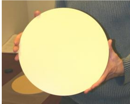
Figure 2. Gradient index lens. The index of refraction is varied radially, enabling a flat plate to focus microwave frequencies. Additionally, the lens is impedance-matched to free space to minimize reflections [11].
