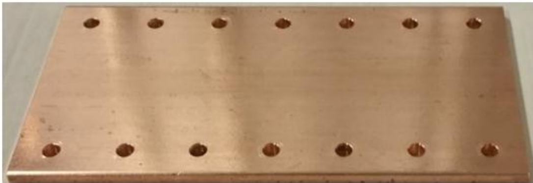
Figure 5-9: Photograph of the coated aerogel plates using a dip speed of 20 mm/min.
