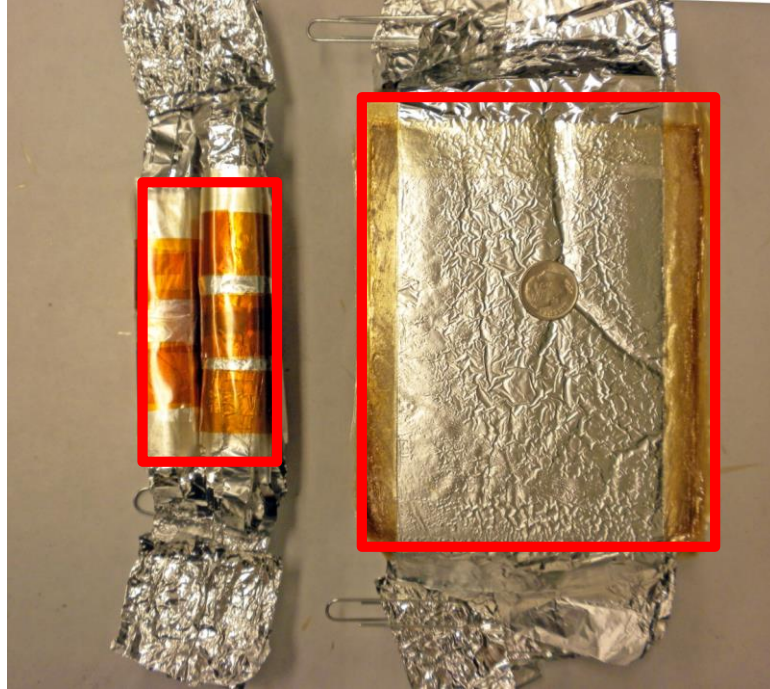
Figure 2. Stacked vs. rolled prototype capacitor volume comparison with dime for scale.
