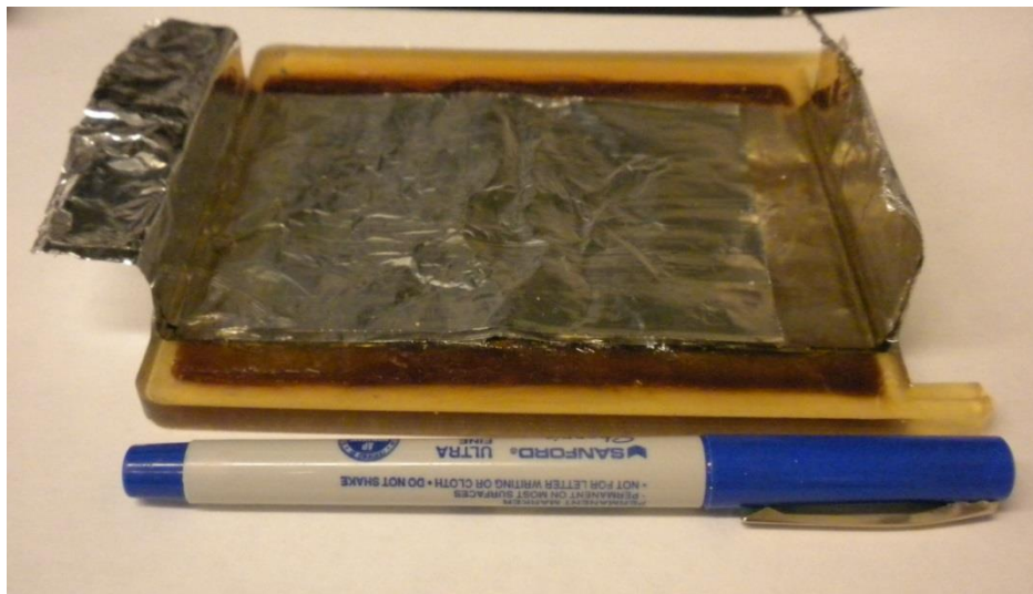
Figure 3. Stacked capacitor potted in epoxy with marker for scale.
