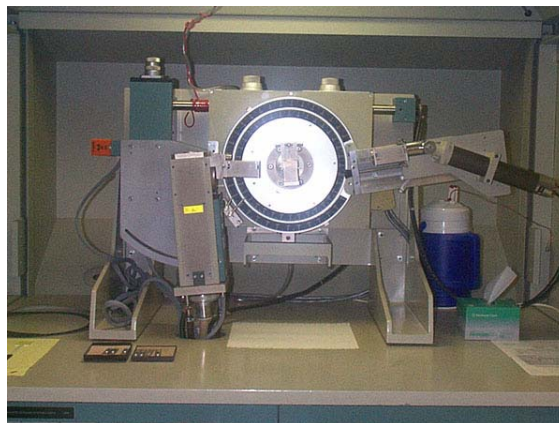
Figure 18 Left: Depiction of the scattered X-Rays giving rise to constructive interference. Right: Image of the XRD machine used at the University of New Mexico.
