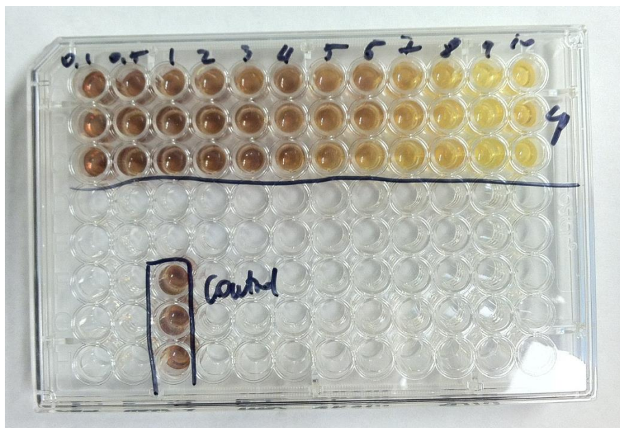
Figure 2.16 Photograph of a 96 well plate after MTS assay was performed for a concentration gradient experiment. The marking 0.1 to 10 denote concentrations of pNIPAM dissolved in cell culture media ( \mu\text{l}/\text{mL} ). “Control” stands for cell culture media without pNIPAM, and “cp” stands for cpNIPAM.
