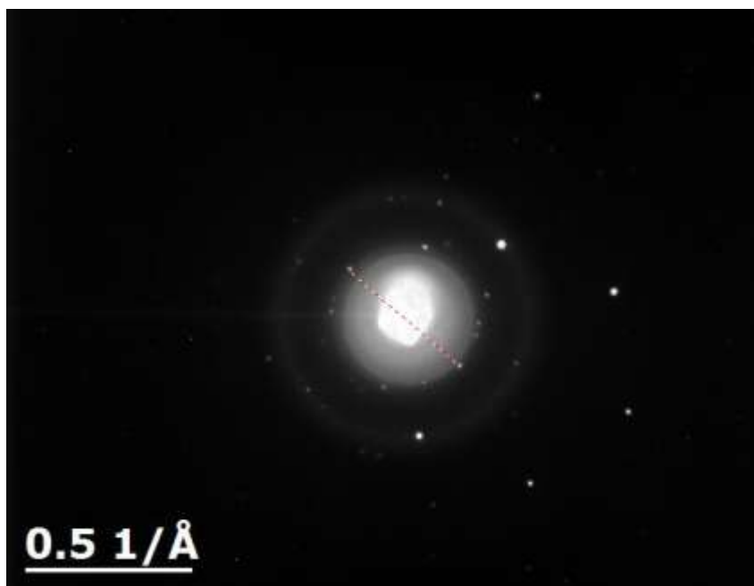
Figure 20. Electron diffraction pattern showing a covered Pt/SiO 2 sample after aging at 800°C for 1.5 hr. The dotted line gives a d_{111} of 2.27Å, the interplanar spacing of Pt.
