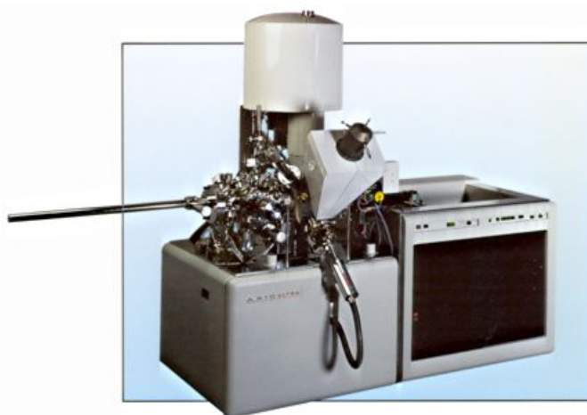
Figure 2.7: A Kratos Axis-Ultra DLD spectrometer.
