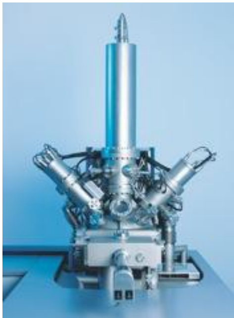
Figure 2.8: An IonToF ToF-SIMS 5 spectrometer.
