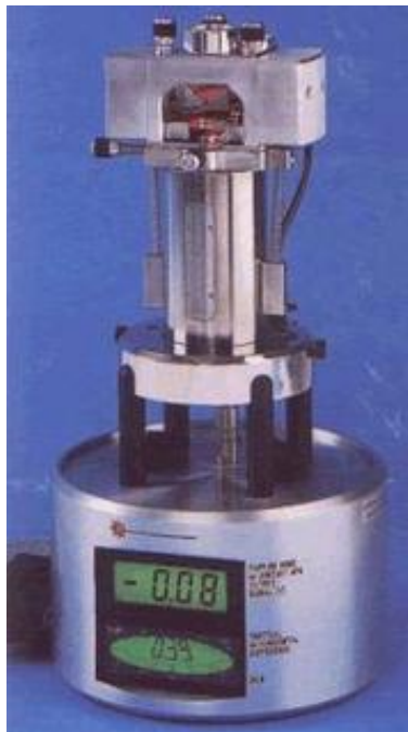
Figure 2.13: A Veeco Nanospec AFM.
