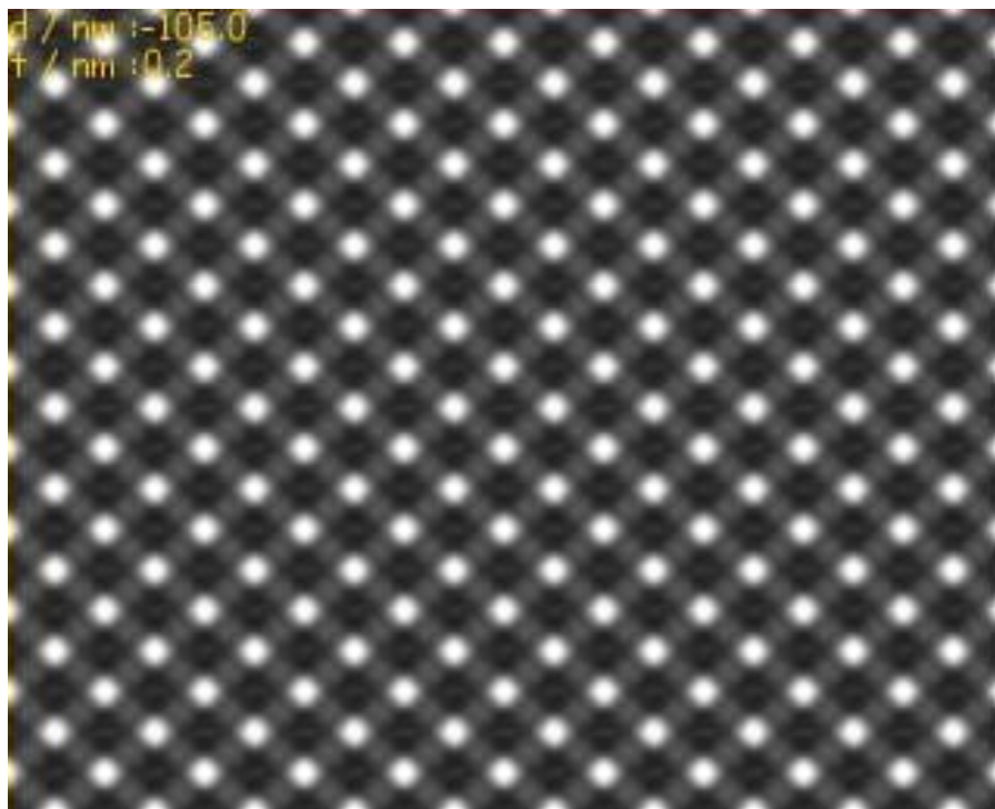
Figure 4.10 TEM simulation result of Fm\bar{m}m structure along [110] orientation.
