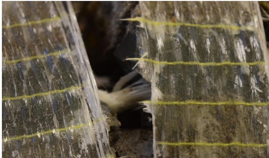
Figure 4.40: Figure showing tension rupture of GFRP bar at failure
