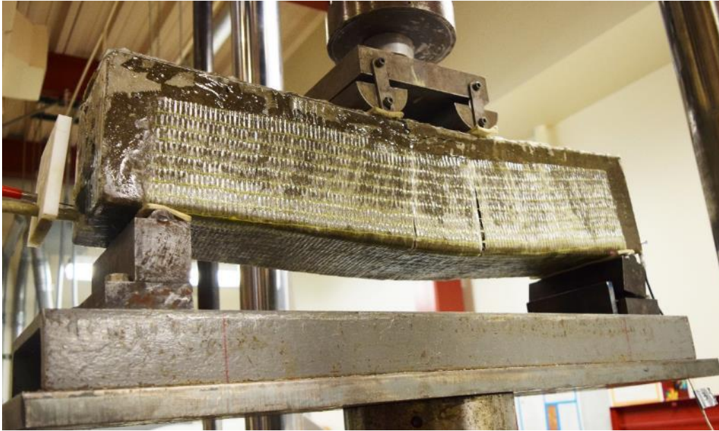
Figure 4.34: RC Beam flexurally strengthened with NSM-FRP and shear strengthened with U-wrap FRP Showing flexural cracks while loading of the beam
