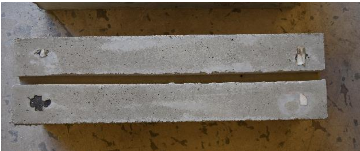
Figure 3.7: Beam NSM groove after cleaning
