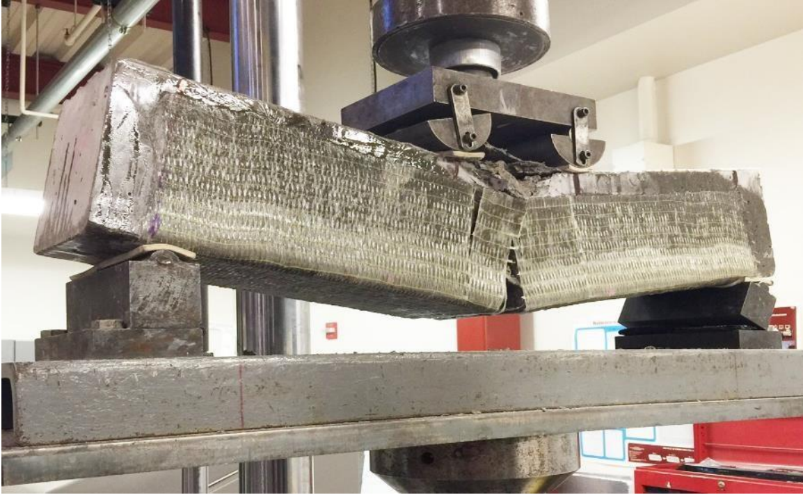
Figure 4.16: RC Beam U3 after failure
