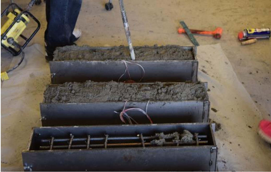
Figure 3.6: Concrete compaction using vibrator
