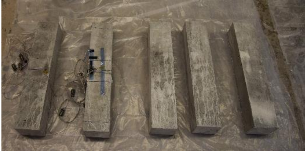
Figure 3.19: Beams control C1 through C5 ready for testing
