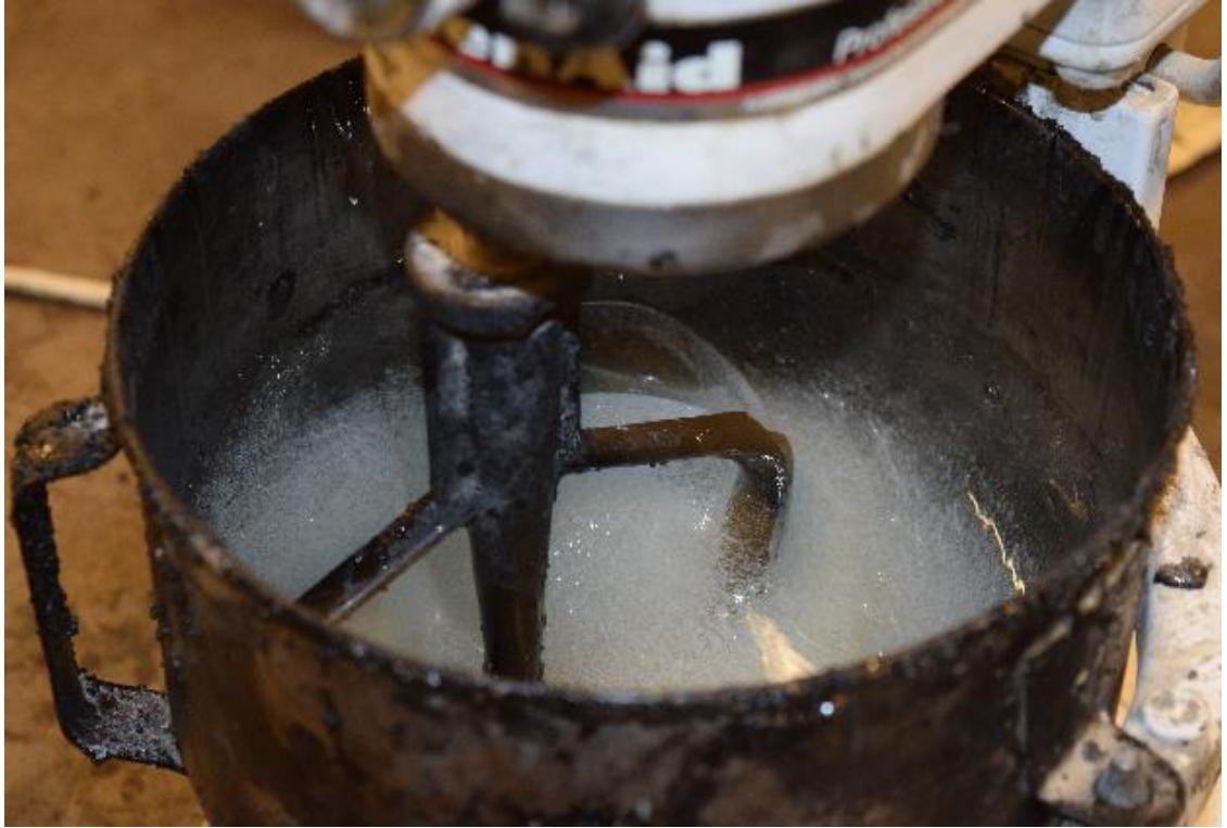
Figure 3.12: Mixing of epoxy for wet-layup
