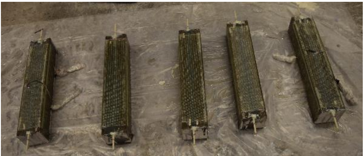
Figure 3.22: Beams with NSM flexural strengthening and U-wrap shear strengthening NU1-NU5 before testing
