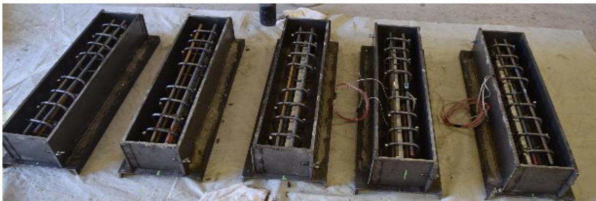
Figure 3.5: Prepared molds before pouring concrete
