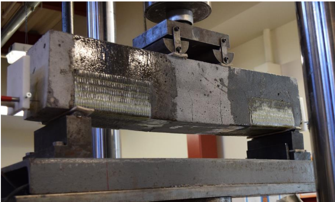
Figure 4.41: RC Beam flexurally strengthened with NSM-FRP and shear strengthened with U-wrap FRP in shear zone only showing flexural cracks while loading of the beam
