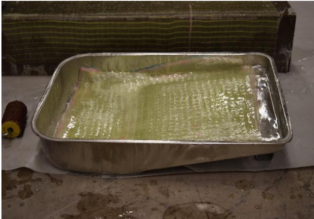
Figure 3.14: GFRP fabric saturated in adhesive
