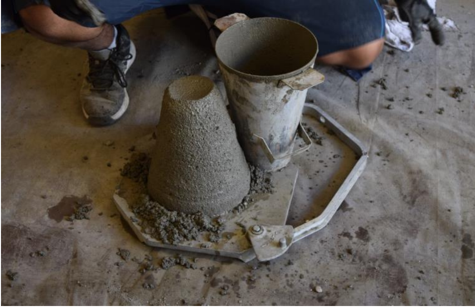
Figure 4.1: Slump of concrete
