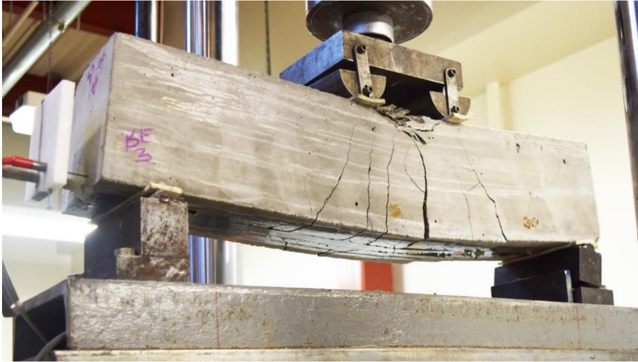
Figure 4.21: NSM-FRP beam post failure showing crushing of concrete
