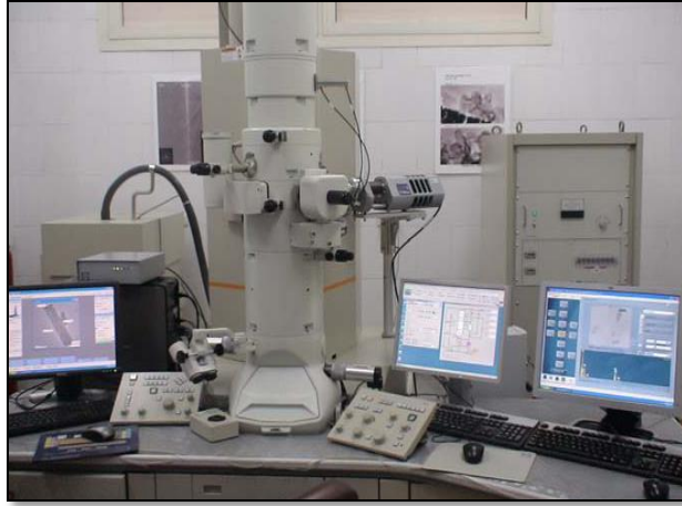
Figure 3.22: JEOL 2100F Transmission Electron Microscope apparatus.
