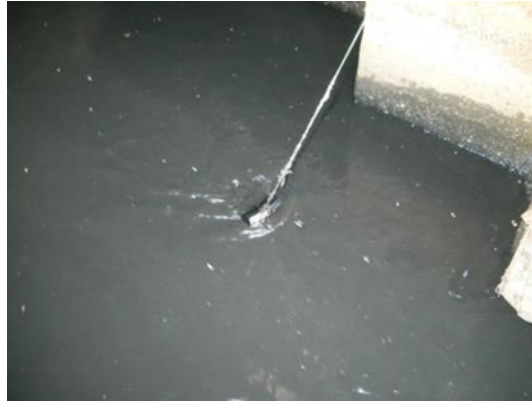
Figure 29 Sample Hanging in Effluent Channel
