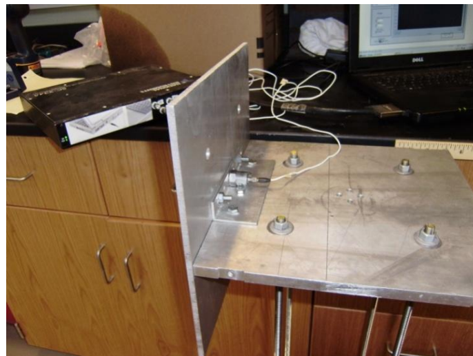
Fig. 7.3 : Vibrational System With Plates Fixed Normal to Each Other. Assuming Large Air-Damping Effect.
