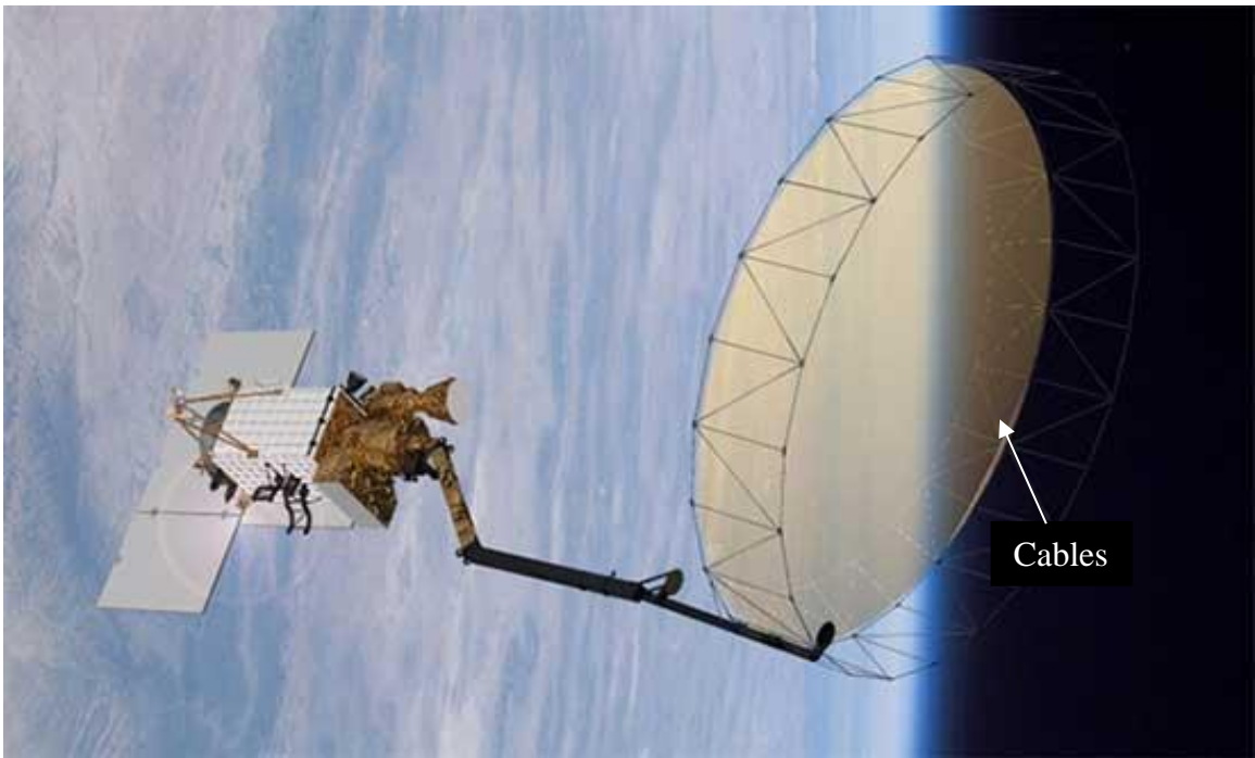
Figure 1.1.2 AstroMesh deployable satellite reflector (Northrop Grumman Corporation)
