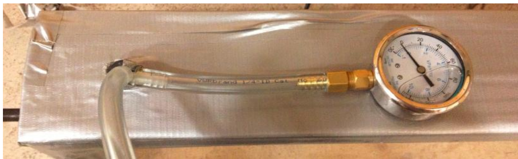
Figure 3.4.4.4 Connection between pressure gauge and chamber
