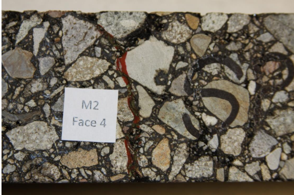
Figure 6.8 Fatigue Cracking in HMA Beam Sample SP-III-M2
