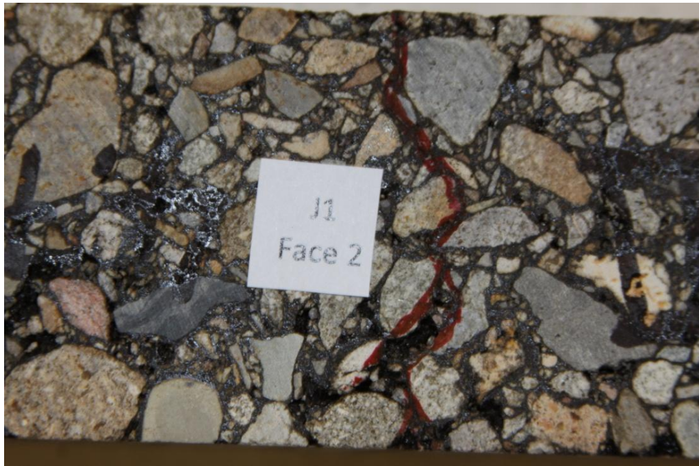
Figure 6.7 Fatigue Cracking in HMA Beam Sample SP-III-J1
