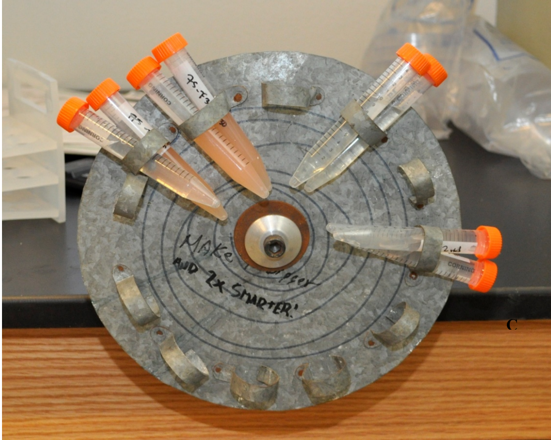
Figure 18: Final experimental preparation. a) Individual test container with septum and needles to gas solution, b) gassing of experiment to achieve desired P_{CO_2} , and c) rotation device to ensure full mixing during experiment.
