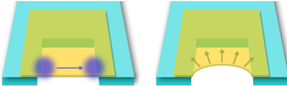
Figure 1 Schematic showing the E-beam irradiation of free-standing nanoparticle/polymer array and the resulting retraction
