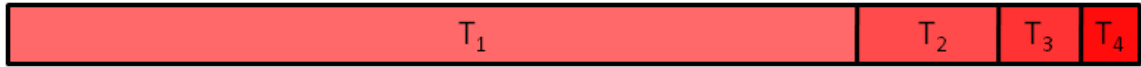
Figure 28: Three-step temperature profile (i.e. four different temperature regions) applied to a 150 m fiber seeded with 16 mW showing the relative lengths of the fiber segments.
