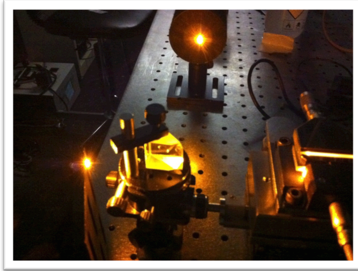
Figure 46: Picture showing output light from a single pass PPKTP crystal to demonstrate frequency conversion to 589 nm signal.
