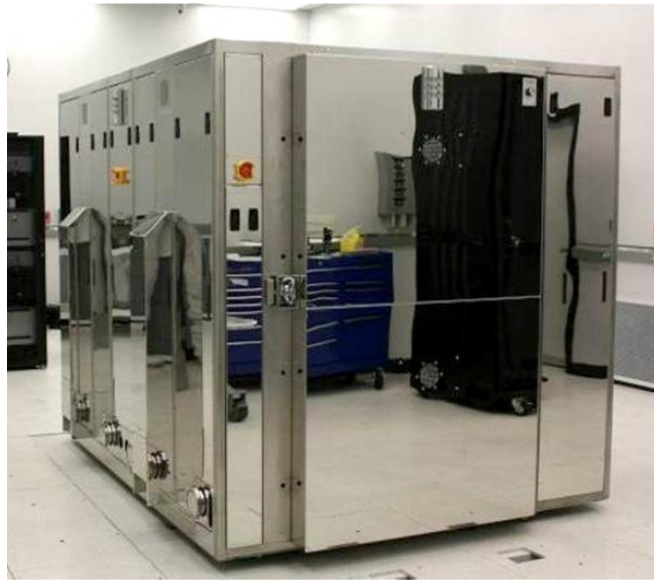
Figure 1: Laser system enclosure for a 7 channel, coherently combined, slab laser system for an output of 100kW [3].
