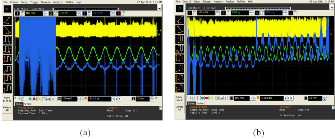
Figure 5.8: OPO pulse train and electrical signals monitored on a digital oscilloscope. Yellow trace is the OPO pulse train at 1200nm, green trace is the modulating voltage on the piezo, and blue trace is the signal obtained from the differential amplifier followed by DC amplifier. The piezo is modulated at different frequencies 11 Hz (a) and 22 Hz (b).
