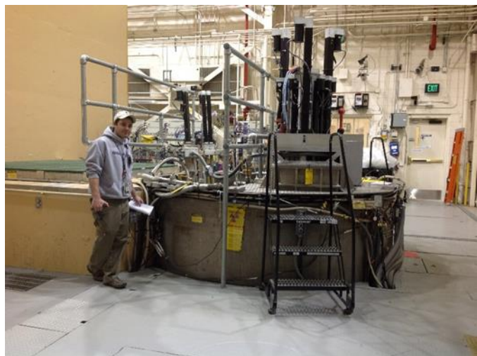
Figure 3 - View of the rod control drive motors (and me) surrounding the opening for the central cavity
