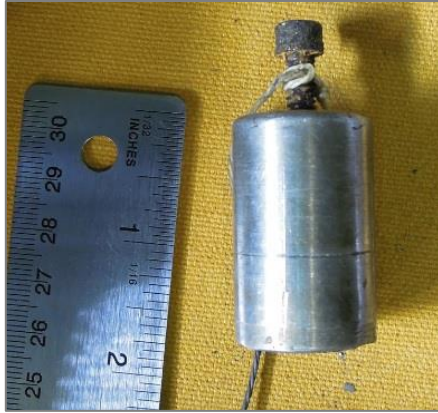
Figure 3. MRC-AmBe-44 Source Photograph and Schematic
