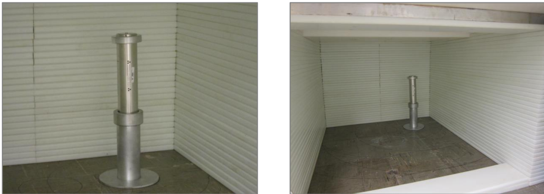
Figure 5. Special Form Capsule on Aluminium Stand inside the Shielding
