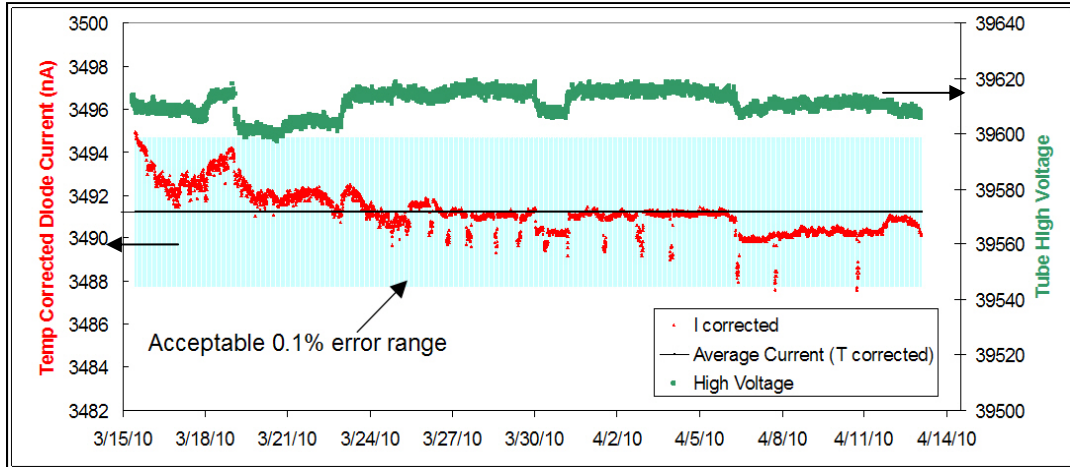
Figure 5-1: Long-term irradiation test of the flux monitor diode at 40 kV and 1 mA. Temperature-corrected diode data are shown, plus high voltage, to help explain the remaining fluctuations.
