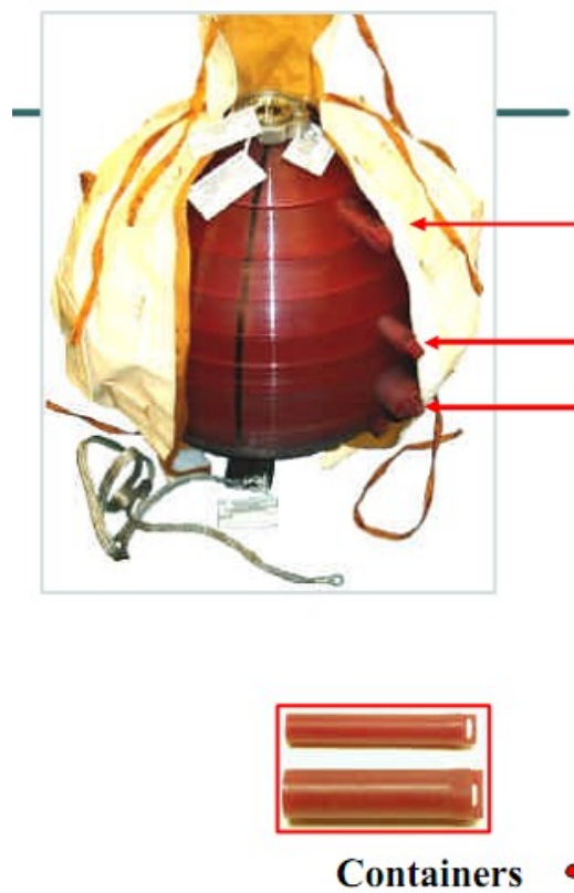
Figure 7.3. Picture of actual phantom with sample detector containers [Kartsev et al. 2005].
