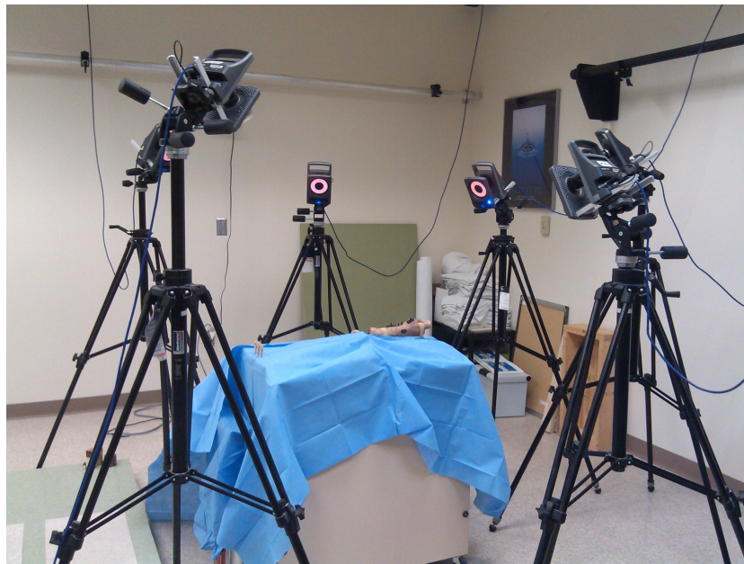
Figure 3.8: Vicon camera system positioned for testing. Six cameras were used to track the motion of all surface markers placed on the specimen.
