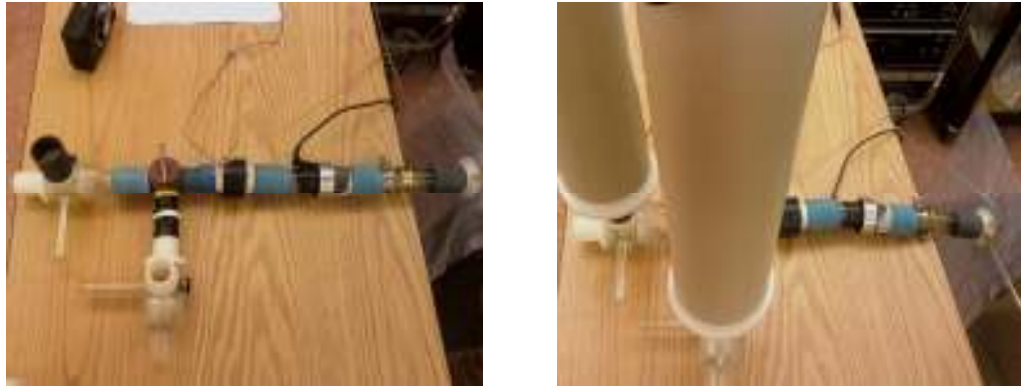
Figure 18. Photograph of the adjusted lung model to suit profiling of changes in inspired and expired gas variables during inspiration and expiration.
