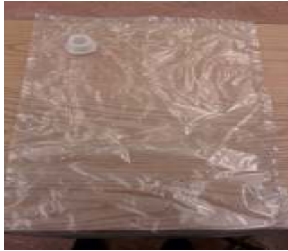
Figure 4. Photograph of the 25 L expired breathing bag used as a small Douglas bag.
