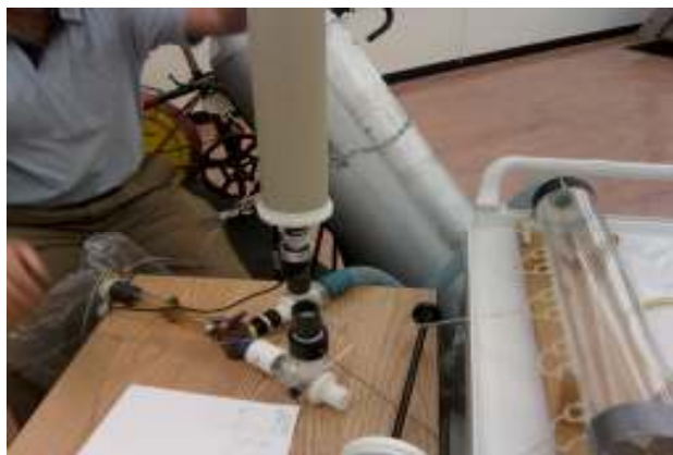
Figure 9. Photograph of the equipment set-up for hypothesis 2 testing for the 5 L fixed volume mixing chamber and expired tubing.
