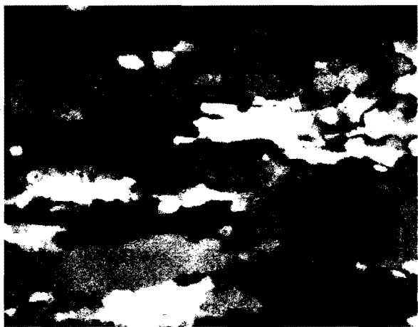
Figure 10: SEM images and photomicrographs of Monazite grains (top two) and microstructures in X-polarized light and plain light (lower right). Monazite grain has rim and core feature with mean age of ca. 1380 Ma. Undulose Quartz stringers with mantle/core microstructures are observed. Images courtesy of Williams, unpublished data.
