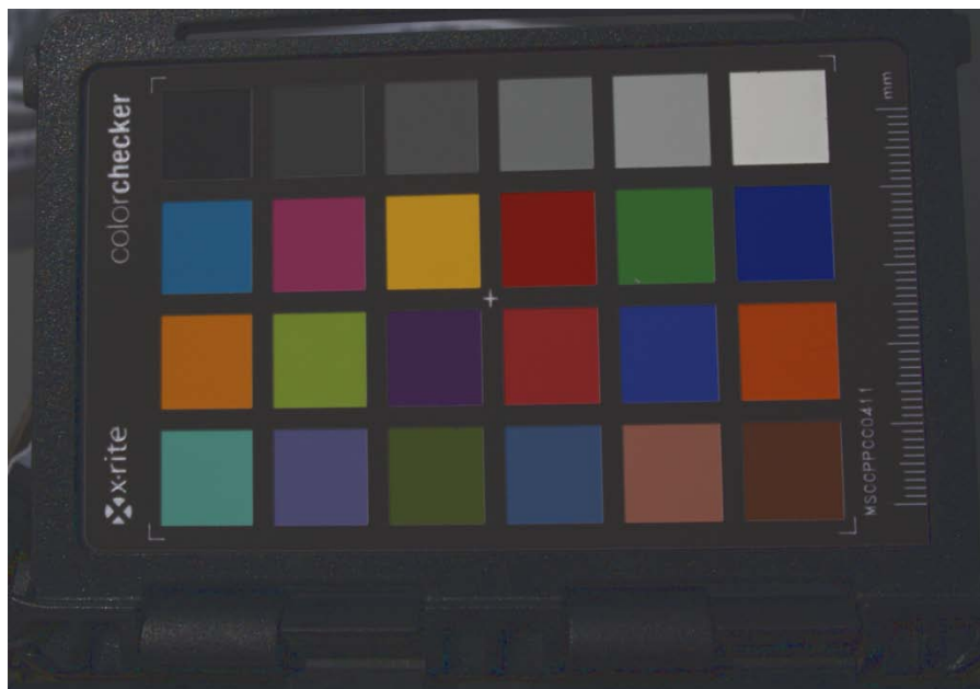
Figure B3. X-Rite ColorChecker Passport reference image used during color calibration and for setting the white balance in Set 2 Imagery
