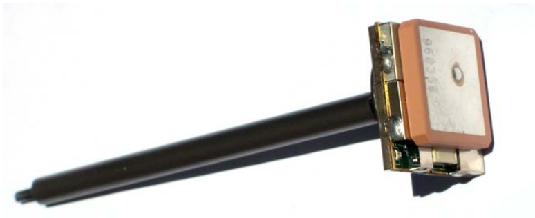
Figure 5 - EM 406A GPS Module attached to aluminum stalk. The threaded end replaces top-plate chassis screw.
