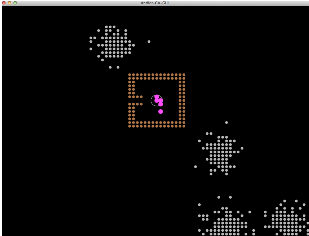
Figure 3.1: The iAnt simulation environment including the bug trap obstacle arrangement and a resource distribution of 256 targets divided into four discrete clusters. Robots are magenta (center) obstacles are brown and resources are gray. The nest is in the center of the trap.
