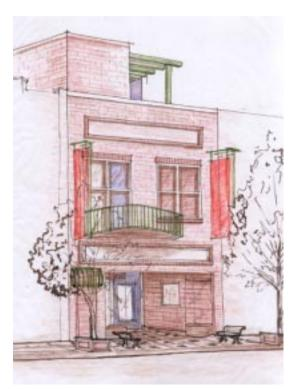
The facade design illustrations provide guidelines for the facades of the buildings on main street. The designs recognise the depth of 10'-14' within the facade in all floors to be a critical volume. Elements like balconies, signage, show windows, skylights, staircases and double height spaces in this volume make the facade dynamic. The sidewalk in front of the stores and street furniture play an important role in integrating the design and creating a unified composition.
