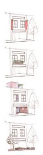
Scheme one shows an internal spiral stairs, a mural wall continuing up all the floors, which along with the trellis, provides shade in the terrace and a curved balcony. The trellis work, balcony and the supports for the signage are proposed to be in wrought iron to subtely compliment the older brick facade.
