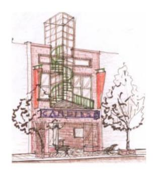
Scheme two shows the building with the spiral stairs to the terrace external to the facade. It has a glass enclosure and is part of the balcony.
