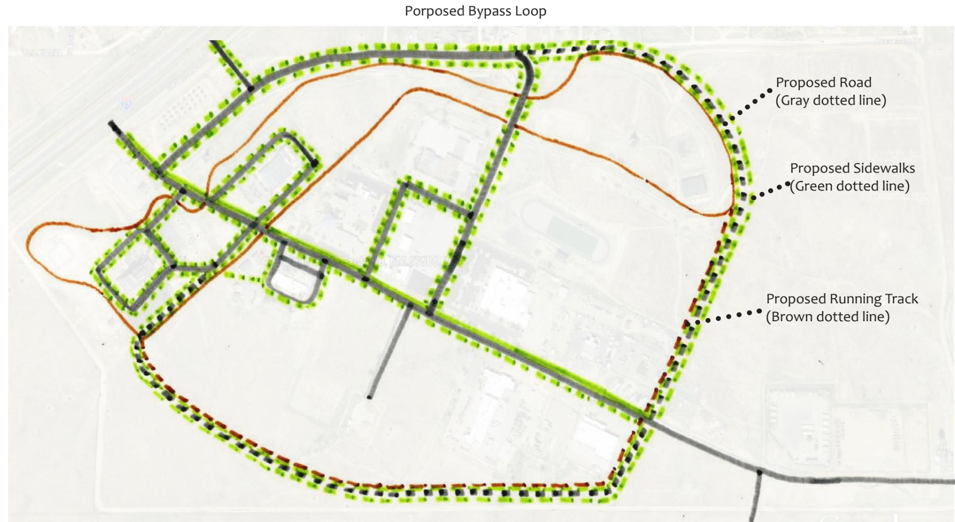
The Oñate Complex Training Site currently has a two-directional layout that connects on the west side of the site with New Mexico State Penitentiary. From a functional perspective, the site is lacking maneuverability; both in a vehicle and on foot. The layout allows one way in and one way out. From an Antiterrorism Force Protection (ATFP) standard, having a loop pattern would enable access to all areas. The NMNG conducts training scenarios regularly which typically require a road
