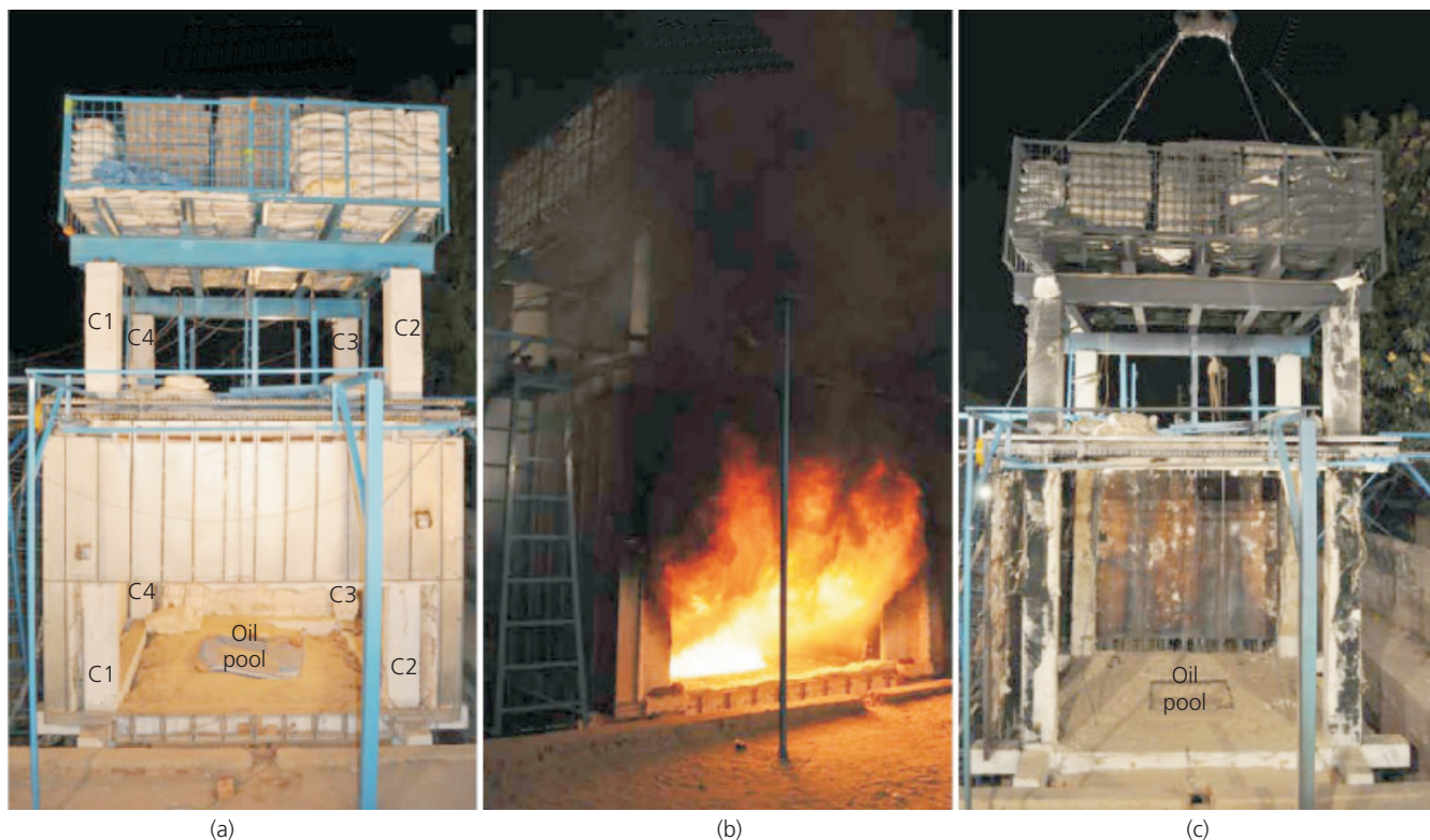
Figure 15. (a) Pre-loaded frame before fire; (b) fire test in progress; (c) fire-damaged frame after test
