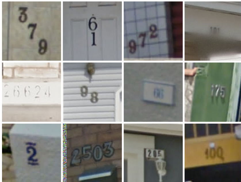
Figure 11.2 – Difficult but correctly transcribed examples from the internal street numbers dataset. Some of the challenges in this dataset include diagonal or vertical layouts, incorrectly applied blurring from license plate detection pipelines, shadows and other occlusions.
