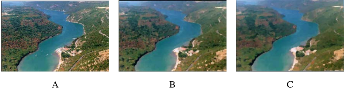
Figure 3.4: (A) The original image. (B) Output of Kuwahara filter with visible blocking effects. (C) Output of [27].
